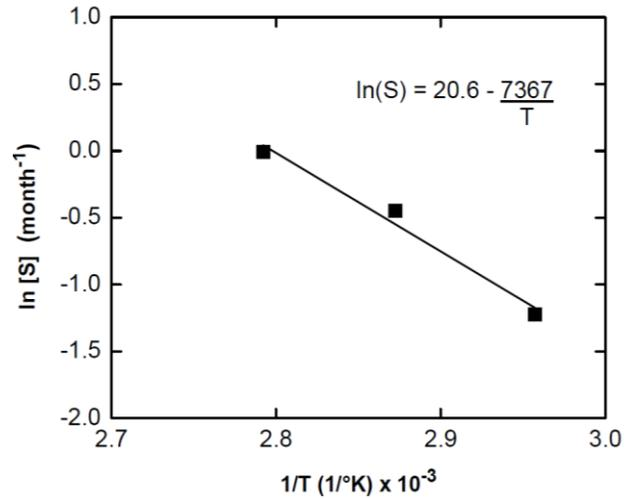
Figure 3. Arrhenius plot of the antioxidant depletion for the GMB immersed in the As-bearing tailings solution.
