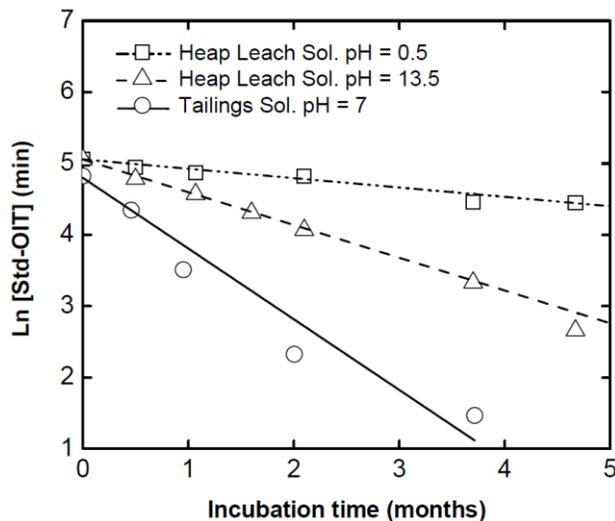
Figure 4. Std-OIT depletion for the GMB examined herein in different mining immersion fluids at 85°C.
