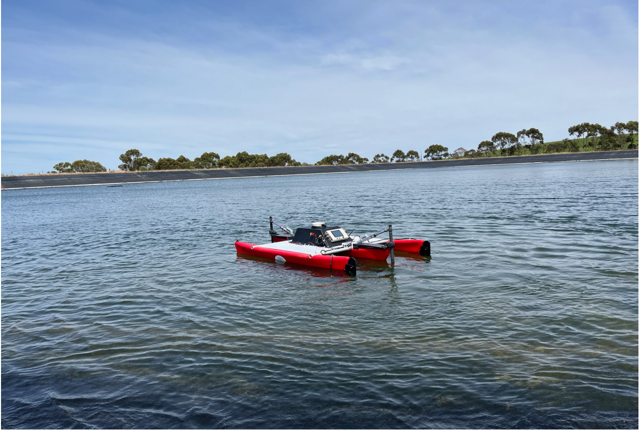
Figure 1. The remote-controlled Geocraft™ Survey Vessel, shown above is surveying a 40,000 m 2 pond, detecting leaks in the geomembrane liner with unmatched accuracy—even at significant depths of 6 m.
