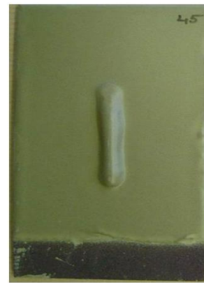
Alkylated Amine Epoxy 2 x 350µm (14 mils)
