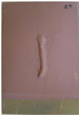
Standard Epoxy Phenolic 2 x 175µm (7mils)
