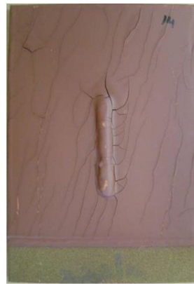
Standard Epoxy Phenolic 2 x 225µm (9mils)
