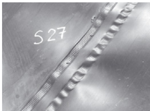
Figure 2 - Example of poor nip roller tracking in a HDPE wedge weld [Scheirs]
