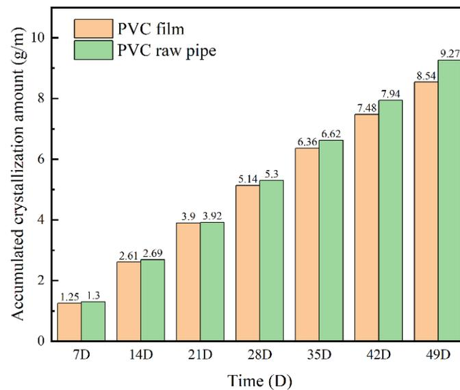
**Figure 3.** Cumulative crystallization of PVC flexible and raw pipes.
