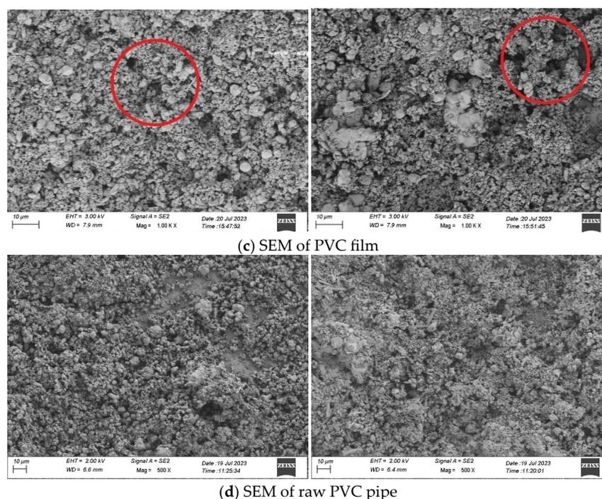
Figure 6. SEM images of crystalline deposits.
