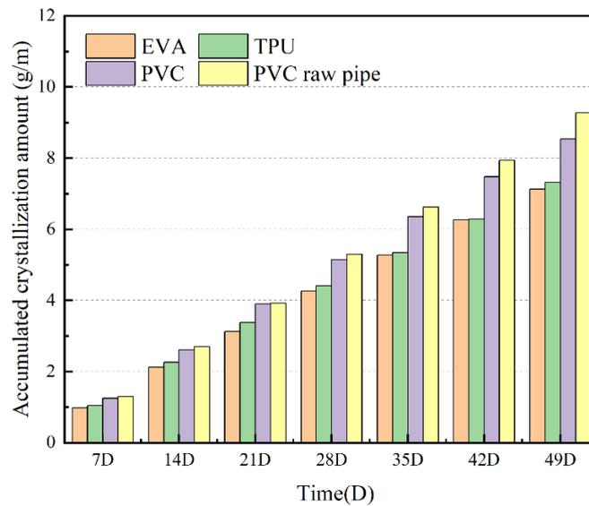
**Figure 5.** Increase in cumulative crystallization in pipes of different materials.
