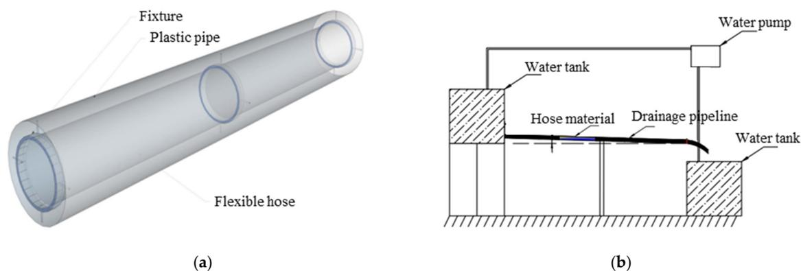
**Figure 1.** Schematic diagram of experimental pipe (a) and schematic diagram of model (b).
