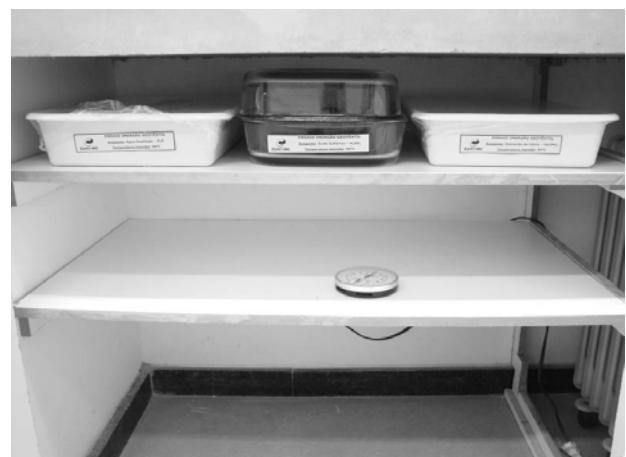
Fig. 2 Sample Immersion at 55°C
