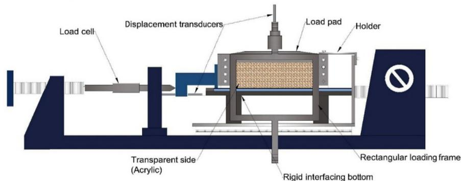
FIG. 2. Schematic diagram of symmetric loading interface direct shear test setup
