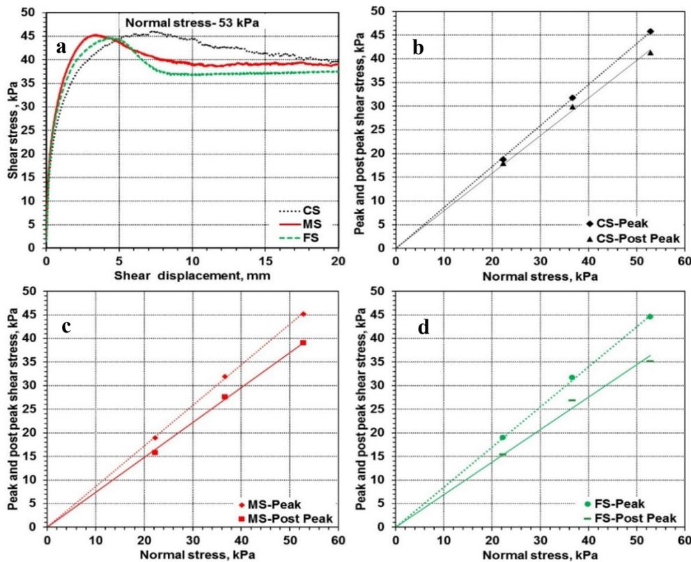
FIG. 3. A representative shear stress-shear displacement and the failure envelopes of the CS, MS and FS
