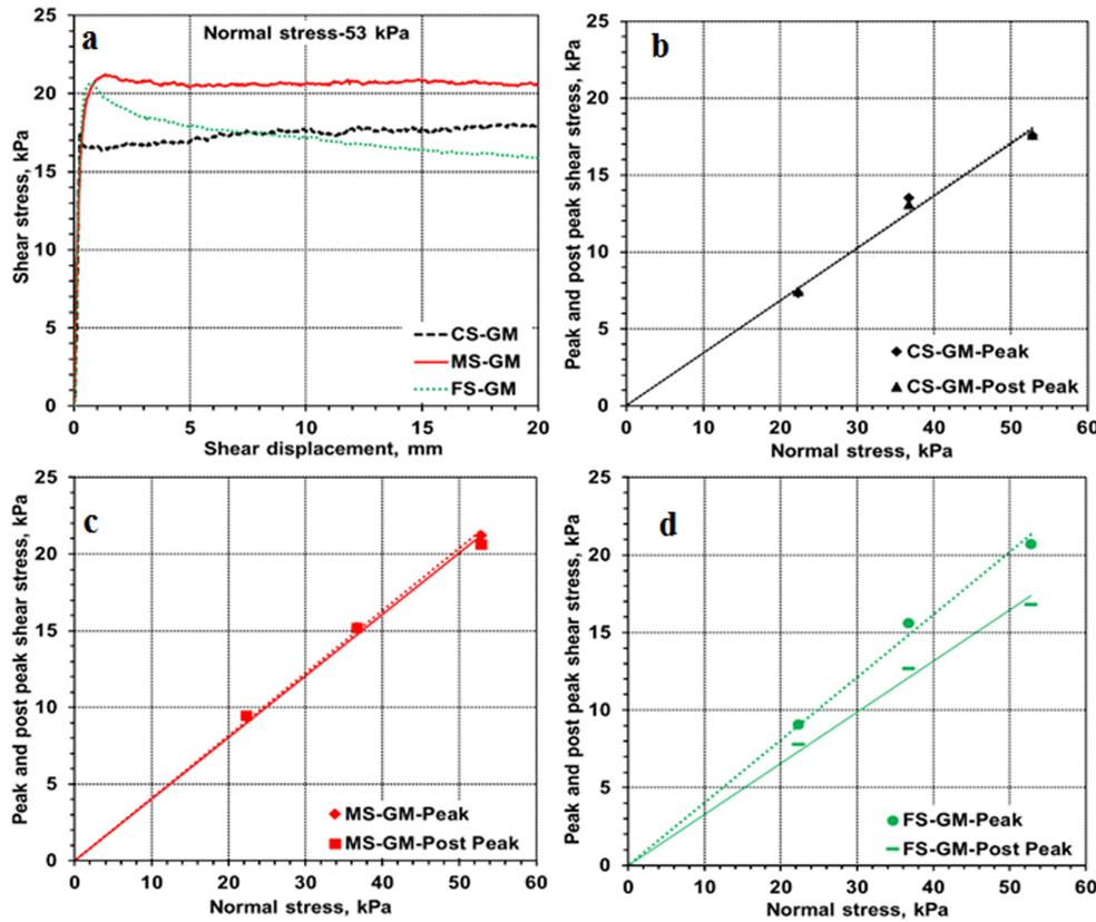
**FIG. 4. Shear stress-shear displacement plots and the failure envelopes for the sand-geomembrane interfaces**
