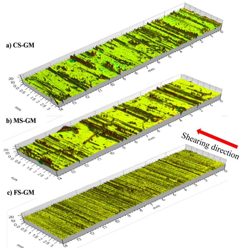
**FIG. 5. Shear induced surface changes on geomembrane by a) Coarse sand b) Medium sand c) Fine sand**
