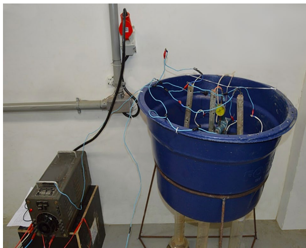
Fig. 2 Electrokinetic dewatering test setup
