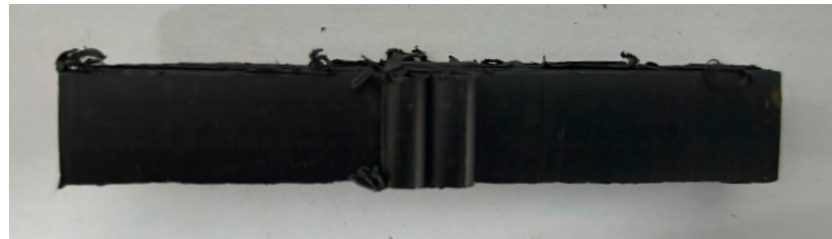
Figure 3. Photograph of a sample for mechanical impact testing.
