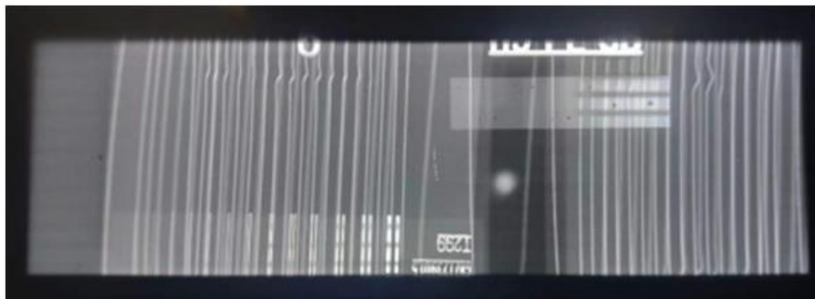
(b) 4# Cold-welding (degree 50%).
