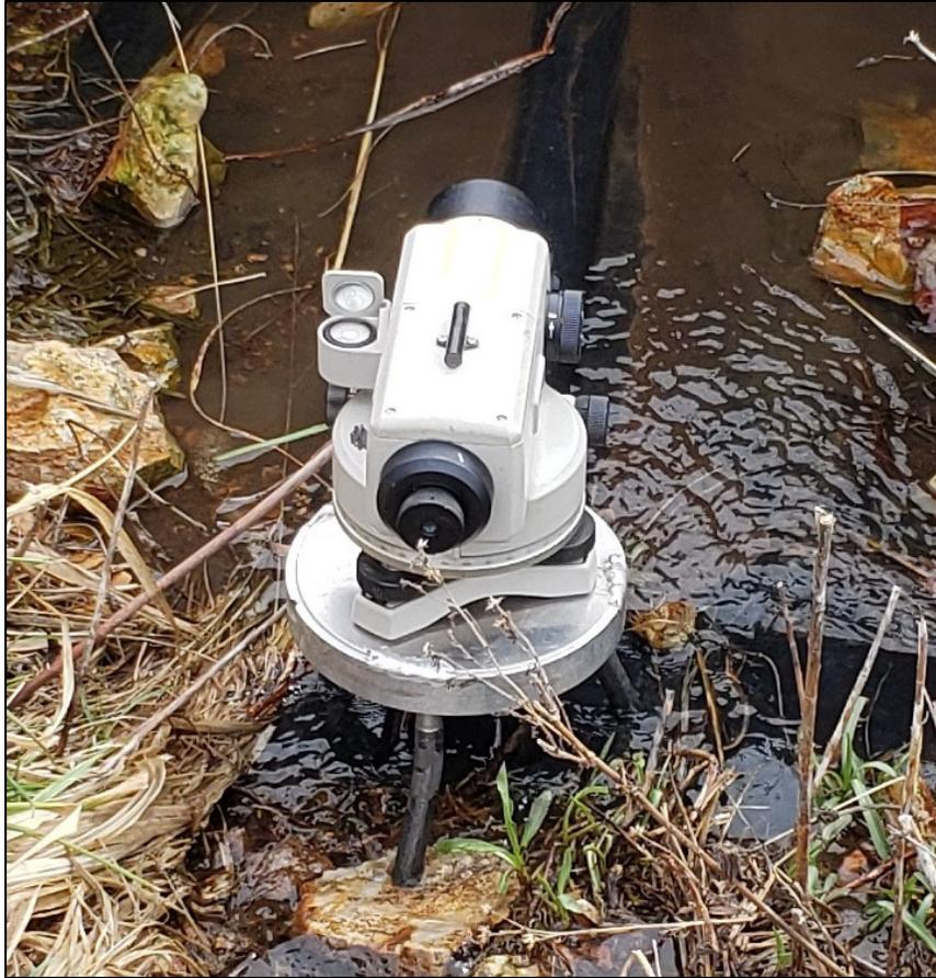
**Figure 5: Level Attached to the Tripod**
