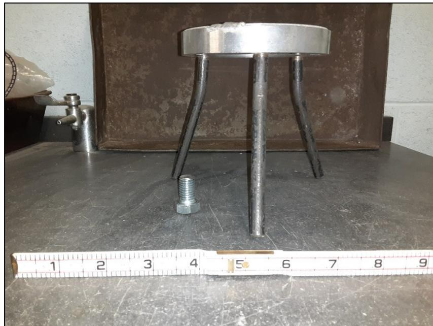
**Figure 4: Special Tripod for Level and Engineers Rule**
