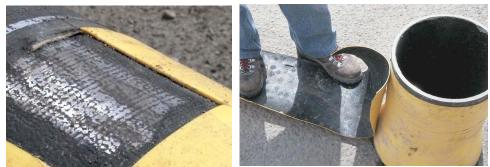
The 'yellow jacket', as shown in the two photographs of Figure 4, above, is a 40mil (1.6mm) thick polyethylene coating which is extruded directly onto the pipe in the factory with a strong bonding agent to permit no gap between. The system was developed for welded oil
