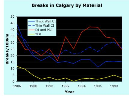
Figure 6. at left, shows the break-rate for Calgary's metallic distribution mains in recent years. DI and PDI are lumped together into one because the PDI on average has only about 30% fewer breaks than "bare" DI, in Calgary's experience. The YDI pipe, with a better coating and cathodic protection, has only 10% the break rate of PDI. The 2-5 breaks/100km/year that do occur, happen at the tiniest breaks in the
