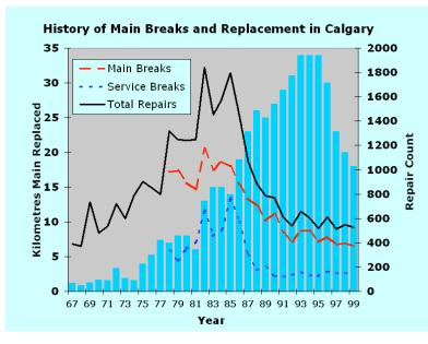
Figure 2, at left, shows the story of Calgary's difficulties with metallic water pipe and part of their response to it. Between 1971 and 1983, Calgary's repairs per year jumped over four-fold, from about 400 to 1600 and even 1800 per year. The rate shocks from the rising repair costs and customer complaints became the major issue facing the utility.
