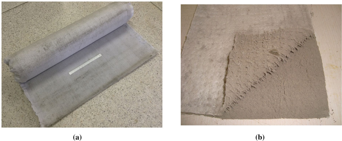
Fig. 1 Geosynthetic cementitious composite mat (GCCM): a a roll of GCCM product; b GCCM's components
