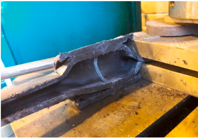
Fig. 8. Shows crushing de-cohesion test on electrofusion joints. Crushing tests showed no considerable differences between appropriately welded and defective joints.
