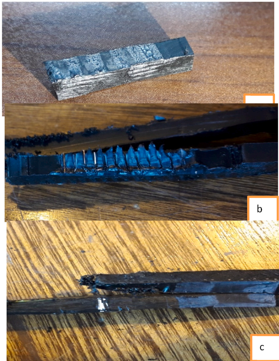
Fig. 9. Optical Macroscopy ( \times 50 ) presentation of fractured surface of the electrofusion welding after strip-bend test containing, (a) improper scraping, (b) humidity, (c) lipid type defects.
