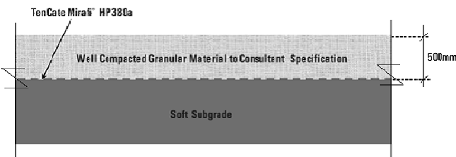
Figure 13 Cross section showing use of Mirafi® HP380a to reinforce the base course aggregates
