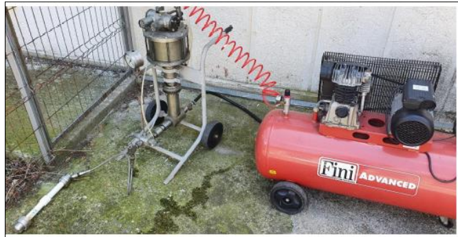
Figure 5. Experimental device used for the burst pressure test
