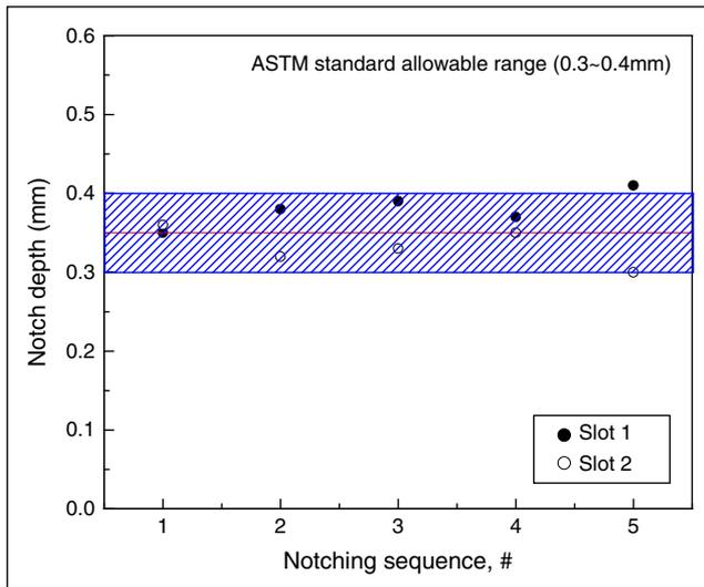
Fig. 10: Variation of notch depth at the center of the fabricated notch with new notcher
