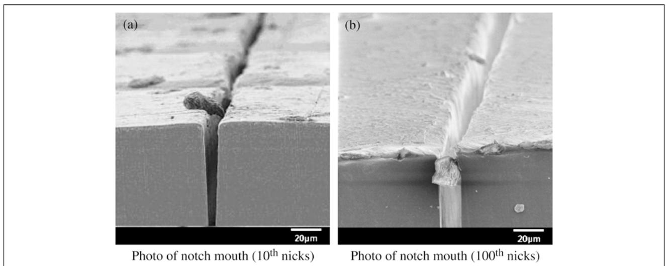
Fig. 5: SEM photos of notch mouth after the 10th and 100th nicks
