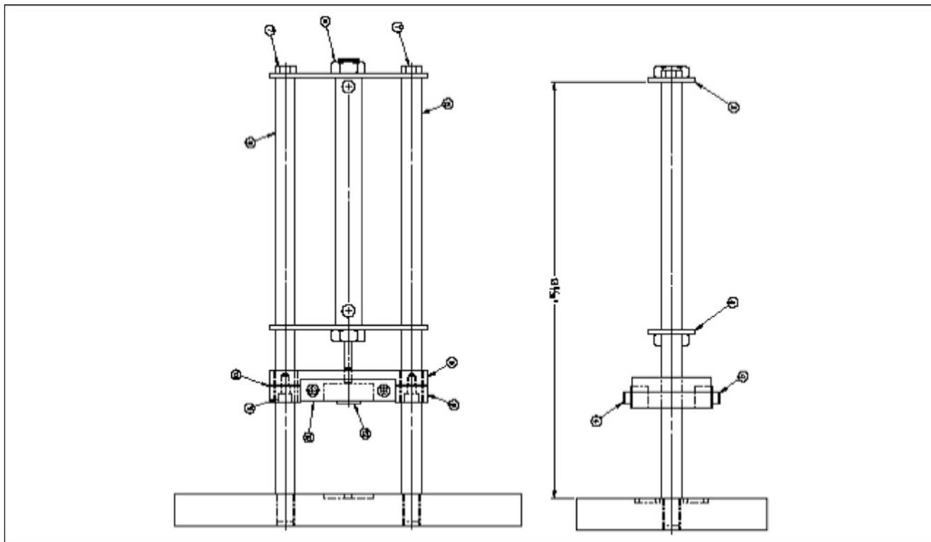
**Fig. 8: Schematic diagram of the newly designed ESCR notcher**
