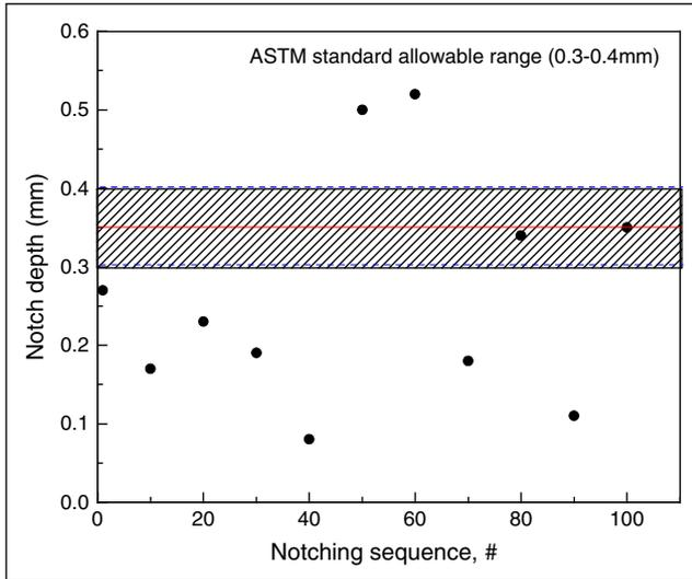
**Fig. 6: Variation of notch depth at the center of the fabricated notch with current notcher**
