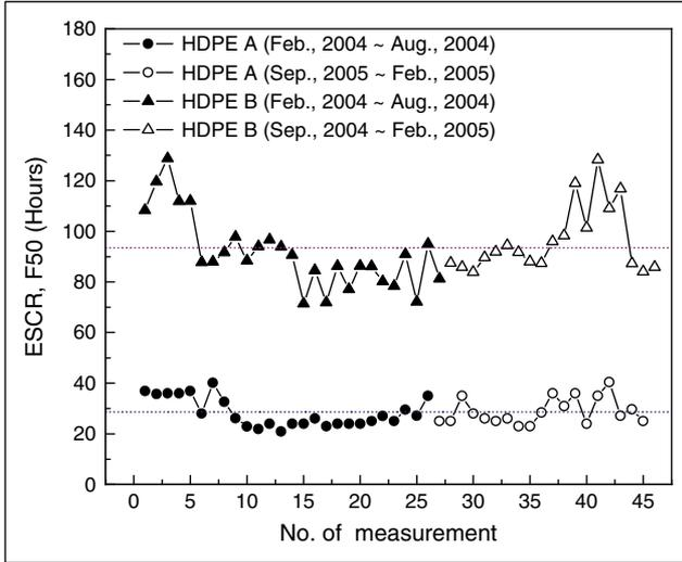
**Fig. 2: Run chart of ESCR measurement variability**
