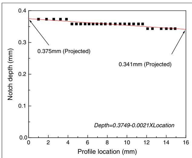
Fig. 11: Variation of notch profile with new notcher
