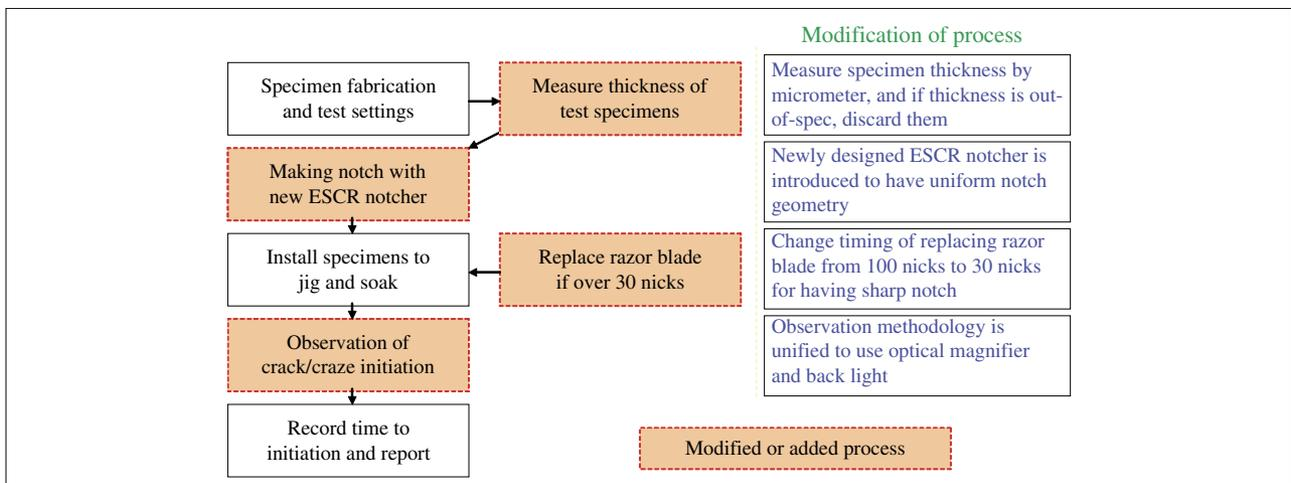
**Fig. 14: Modified process map of ESCR test**
