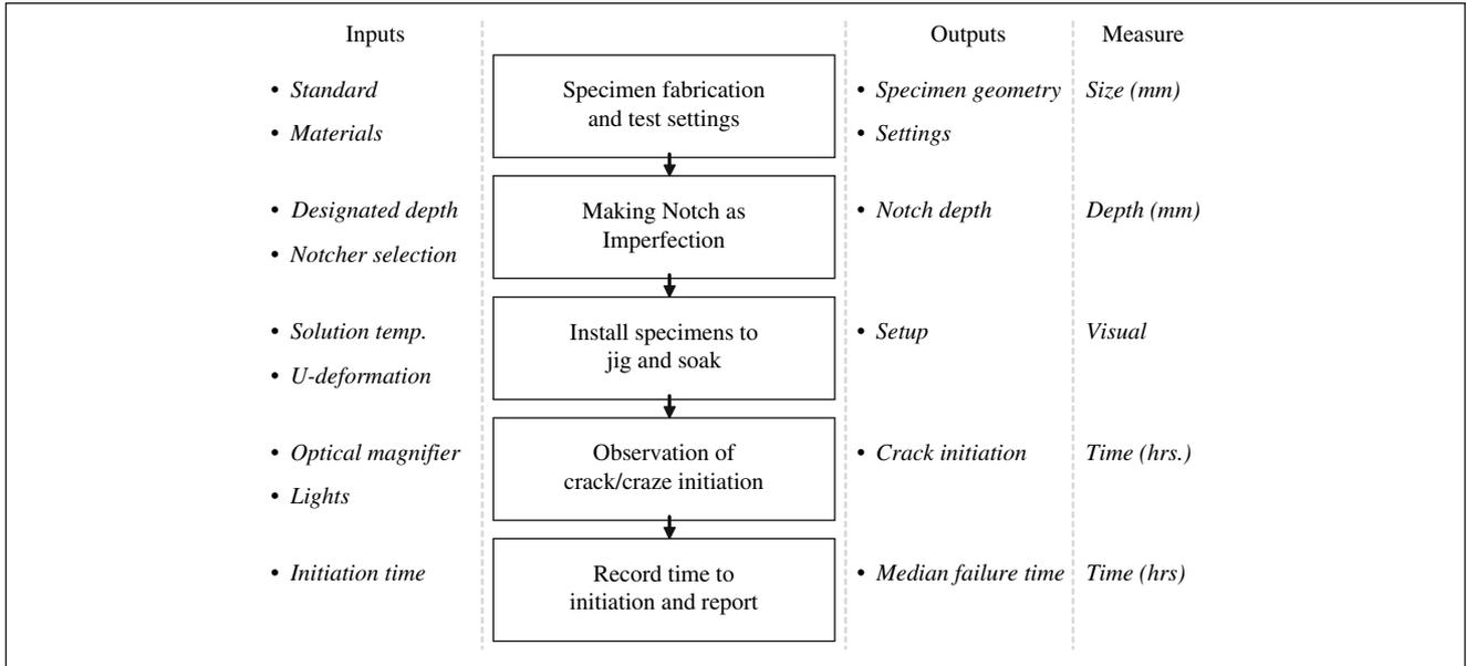
**Fig. 1: Process map of current ESCR test**
