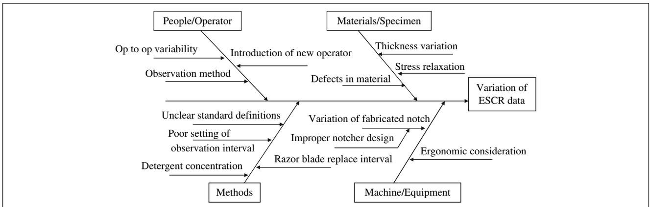
**Fig. 3: Fish-bone diagram for the root cause analysis of ESCR test**
