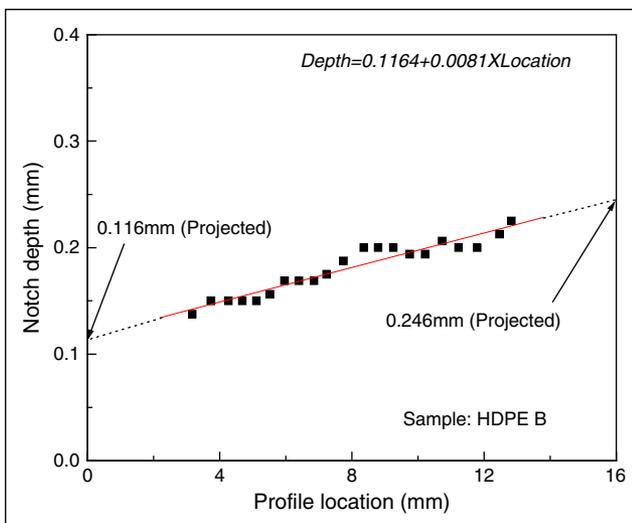
**Fig. 7: Variation of notch profile with current notcher**
