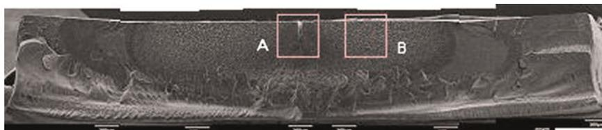
Fig. 12: Fracture surface of ESC
