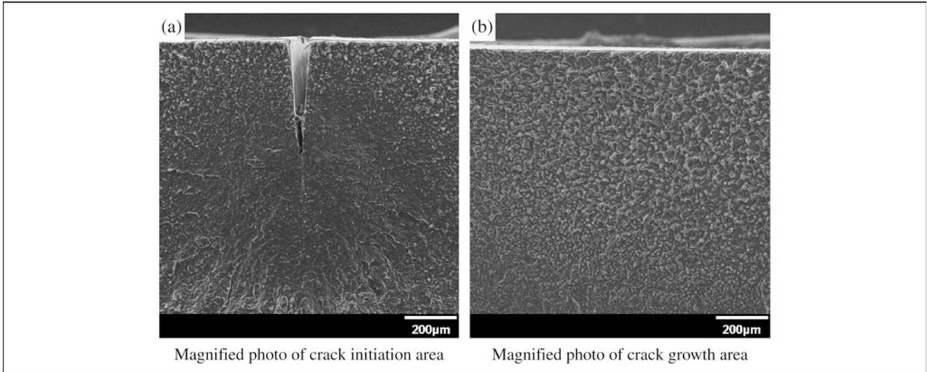
**Fig. 13: Magnified photos of fracture initiation and propagation of ESCR. (a) Magnified photo of crack initiation area and (b) magnified photo of crack growth area**
