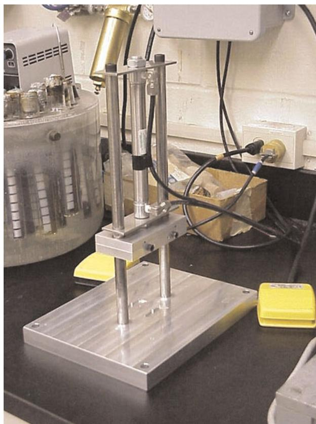
**Fig. 9: Installed new ESCR notching machine**
