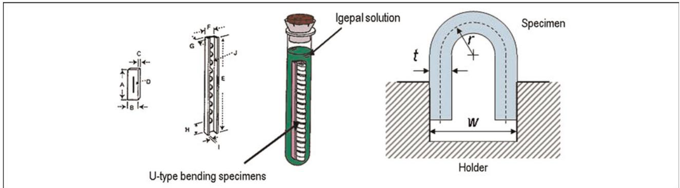
Fig. 4: Strip bent test based on ASTM D1693
