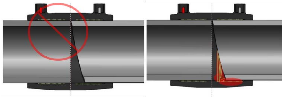
Figure 39: Mis-Cut - Incorrect Assembly
