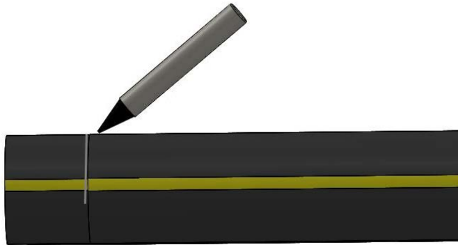
Figure 23: Remark Stab Depth
