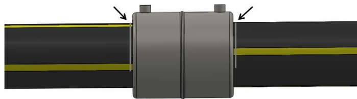
Figure 24: Install fitting to stab depth
