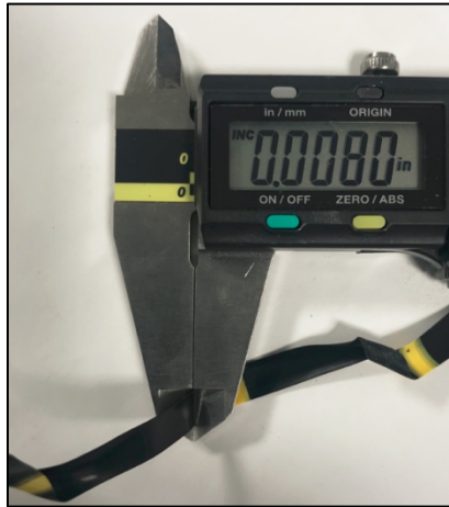
Figure 8: Scraping/Peeling measurement using a caliper
