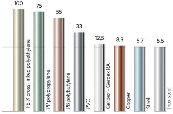
Relative thermal expansion of pipework materials
