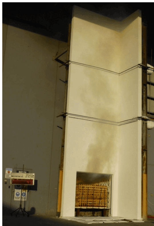
Fire 32 The external wall system during the test – 49 seconds after crib ignition
