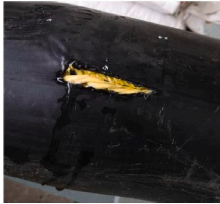
Fig. 20. Example of pipe burst subjected to quasi-static internal pressure with an external lateral dent in an RTP pipe [83].
