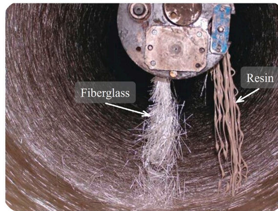
Fig. A.31. An illustration of the centrifugal casting process is shown, providing an inner view of a steel mold.
