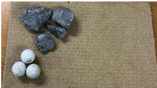
Figure 7.8. Oversized aggregate recovered from the leachate collection system specified as 38 mm to 75 mm aggregate in a 300 mm thick layer above a geotextile cushion or protection layer aimed at limiting geomembrane strain.
