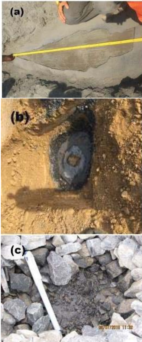
Figure 7.7. Typical construction related problems: (a) Tear induced by material shearing (platinum tailings storage facility); (b) Rotational tear induced by wheel turning; (c) Dust penetration of a geotextile protection layer interface
