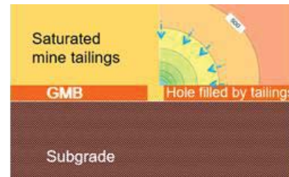
Figure 5.3. A single geomembrane covered by silty sand tailings forms a composite system with the tailings above and within the hole, substantially reducing leakage through the hole. The nature of the subgrade can also control the service life of the geomembrane.
