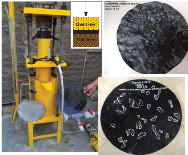
Figure 8.9: Puncture testing device and damaged geomembrane
