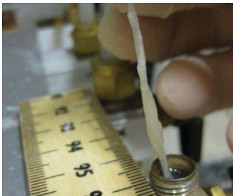
Figure 4.17. Mobile polyacrylate hydrogel crosslinked with \text{Ca}^{2+} eluted from flexible-wall permeameter (note: scale is in mm).
