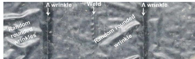
Figure 2.15 Aerial photo of \Lambda wrinkles arising at quarter points from fold in blown film geomembrane running parallel to the roll
