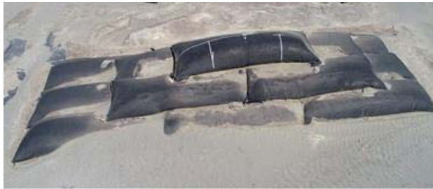
Figure 8.47 Bird-eye view of the drained stacking of geotextile tubes that remained in the field for 24 months.
