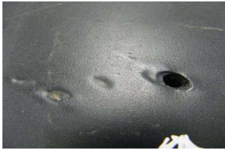
Figure 2.12 Lacing hole defect in an HDPE geomembrane caused by die build-up.
