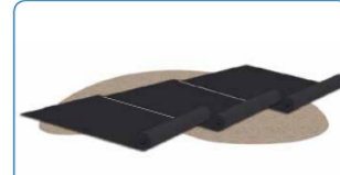
Figure 1: Absolute Barrier Overlapping Roll-out Method
