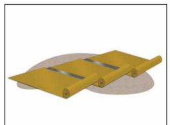
Fig. 1: VaporBlock® Plus™ Overlapping Roll-out Method
