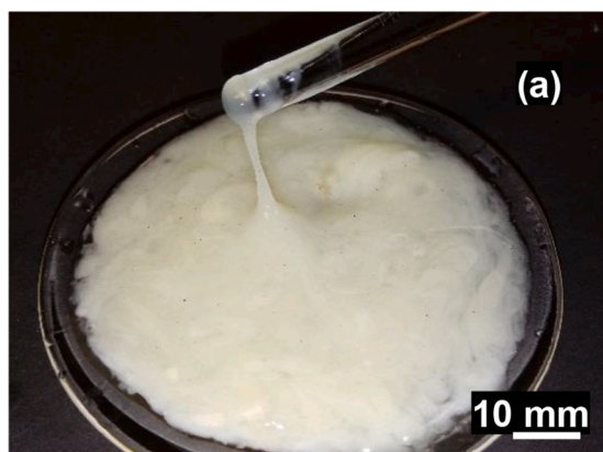
Fig. 7. Images of two different types of polymers found in B-P GCLs: (a) B-P-3.7 and (b) B-P-3.4.
