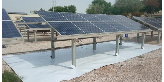
Fig. 2. Photo of experimental PV test-stand, used in this study as an example-validation case, representing regular other validations of our model. In this study, we compare the energy yield of this set-up against an identical system without artificial ground albedo enhancement.
