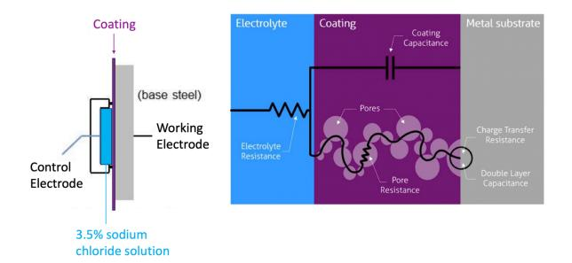
One of the most important factors of protection against corrosion by barrier coatings is through their resistance to ion transport though pores, defects and free volume in the coating and this is what EIS measures. As a guideline of the protective behaviour of coatings the following ranges of impedance denoted as  $Z_{0.1 \text{ Hz}}$  are applied:
