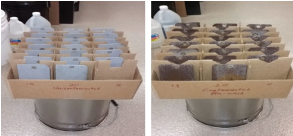
Fig. 1: Control (left) and contaminated panels (right) before preparation. Figures courtesy of the authors
