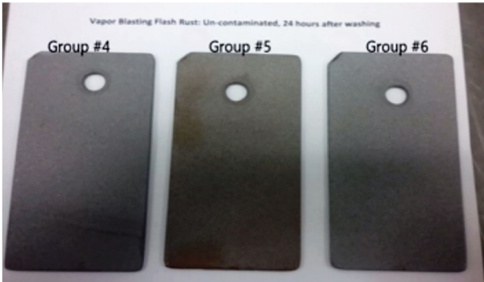
Fig. 3: Flash rust comparison between control panels
