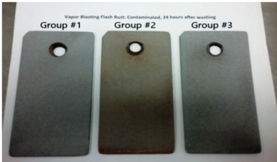
Fig. 2: Flash rust comparison between contaminated panels
