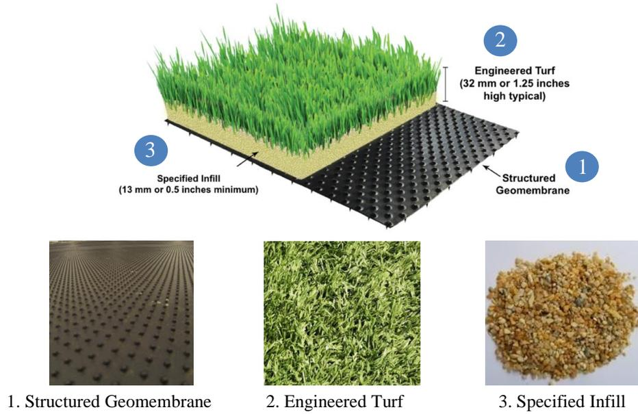
Figure 1. Illustration of engineered turf cover and system components.
