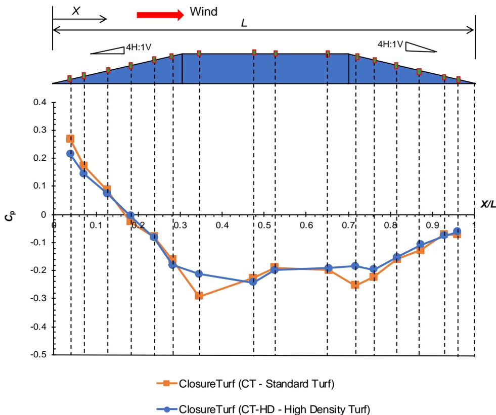
**Figure 7. Wind pressure coefficient distributions of engineered turf cover with 4H:1V slope**
