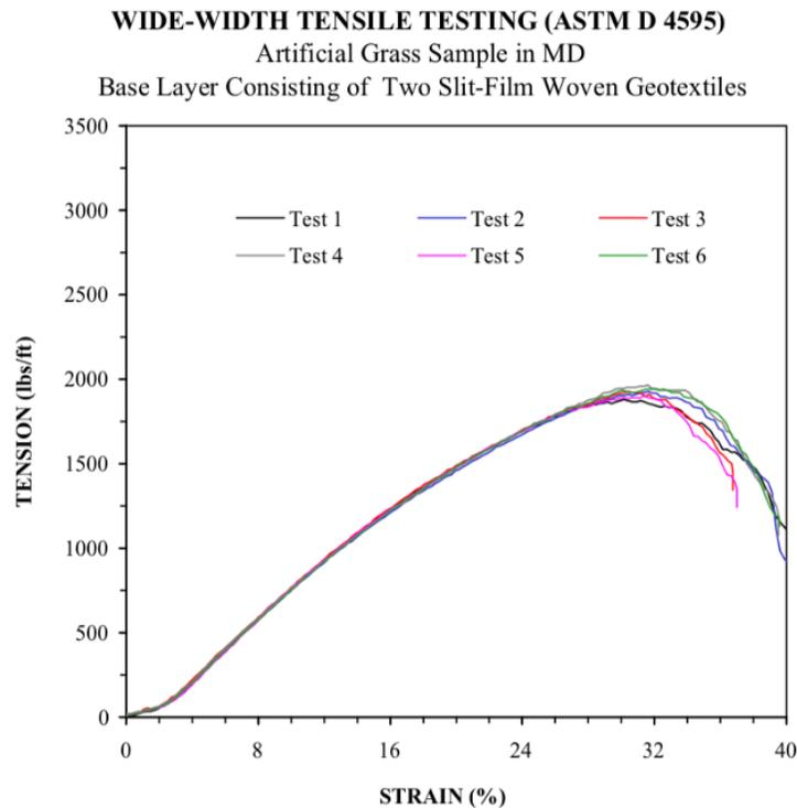
**Figure 4. Tensile test results of engineered turf.**
