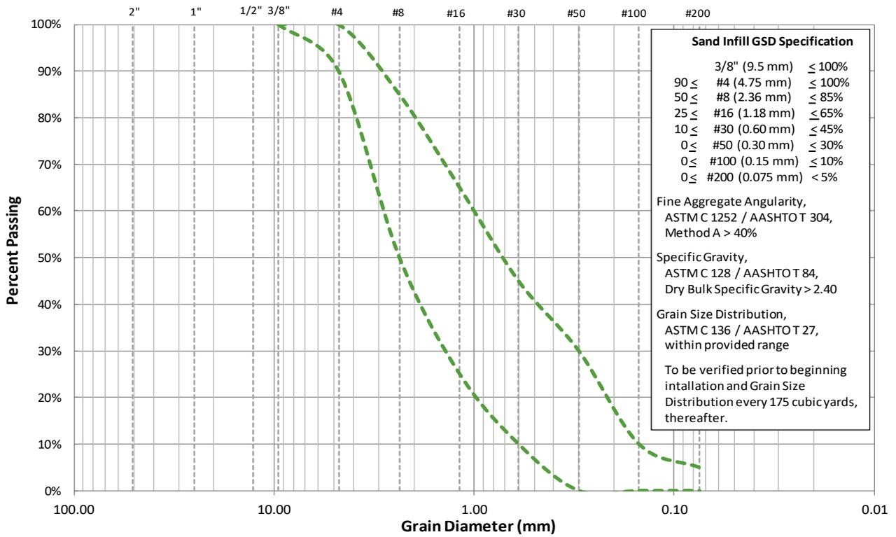
Figure 2. Engineered turf cover sand infill specification.
