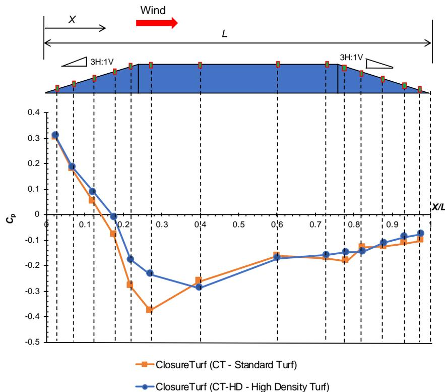
**Figure 8. Wind pressure coefficient distributions of engineered turf cover with 3H:1V slope**
