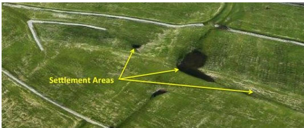
**Figure 5. Differential settlement on engineered turf cover [O'Malley et al. 2017].**
