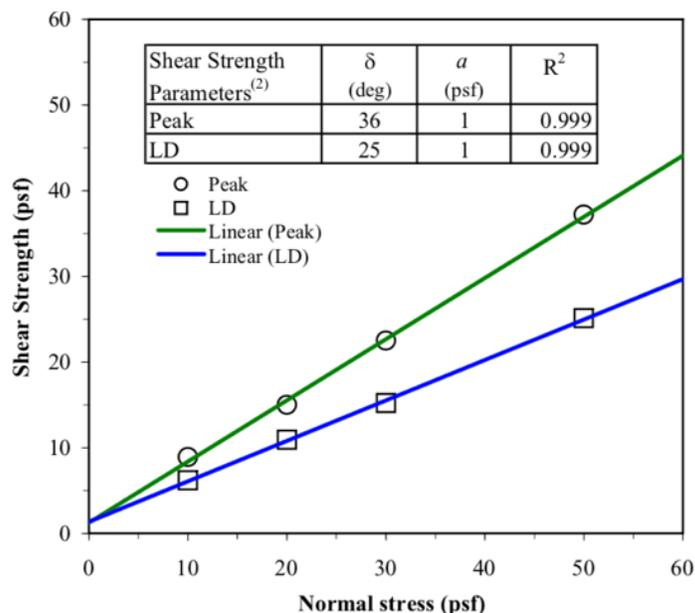
Figure 3. Direct shear results between engineered turf and structured geomembrane.
