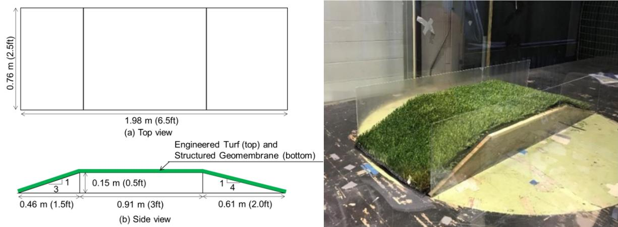
**Figure 6. Engineered turf cover wind tunnel testing.**
