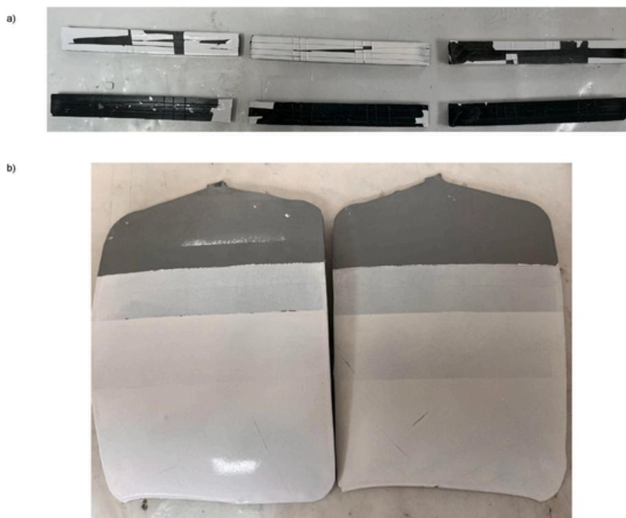
**Fig. 6.** a) Previous coating scheme cross-cut test, from left to right Barnicoat 400E, Novolack and Novoacrylic. Upper schemes being sanded, and lower ones not sanded; b) Final coating scheme cross-cut test, from left to right Novolack and Barnicoat 400E, both previously sanded.
