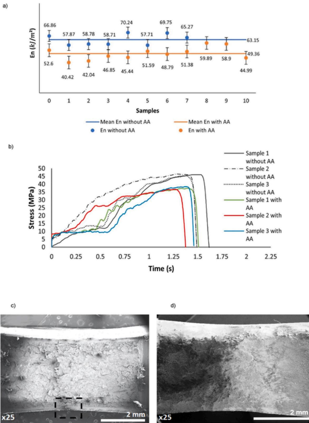
Fig. 5. a) Impact energy absorbed by each specimen; b) Stress vs Time for each specimen; c) SEM micrograph of the fractured region before AA; d) SEM micrograph of the fractured region after AA.
