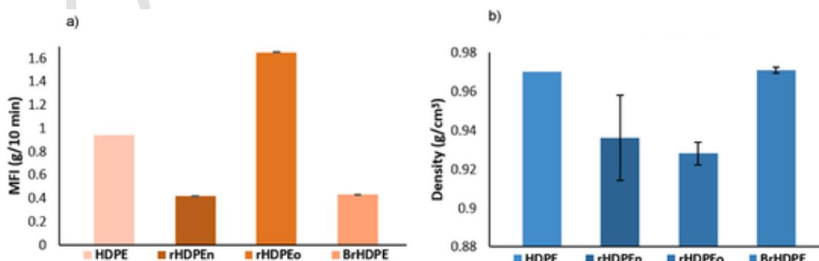
Fig. 4. Test results of: a) fluidity index and; b) density.
