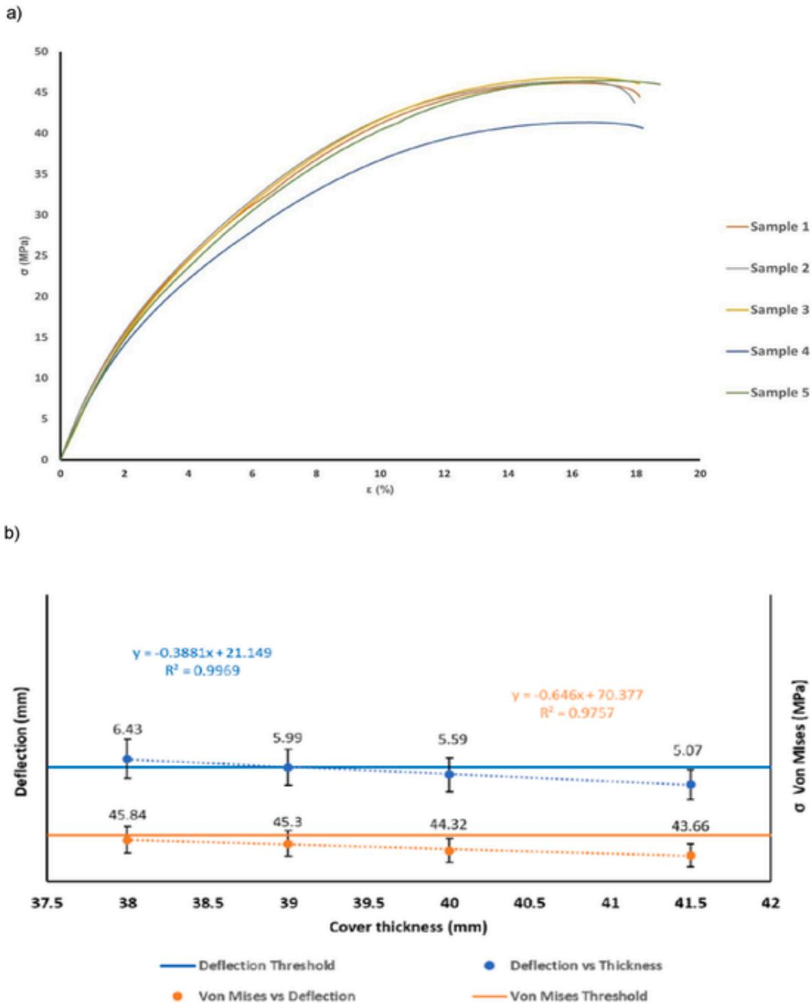
Fig. 7. Numerical simulation results: a) Stress-strain curves for tensile behaviour; b) Thickness verification and maximum deflection.
