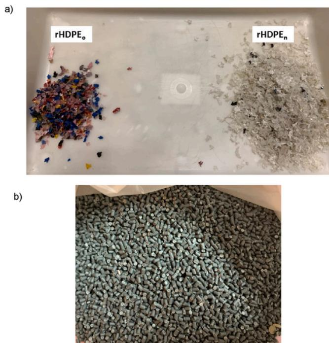
**Fig. 2.** Physical appearance of: a) rHDPE granules before mixing; b) BrHDPE formed with a 3-mm size.
