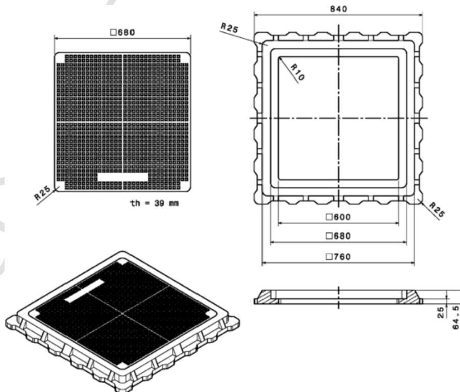
Fig. 3. The 3D Models, including an isometric view and basic dimensions.
