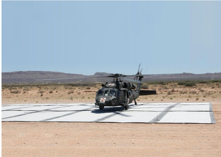
Figure 5. Military Helipad to prevent “brown-outs” from rotor wash.
