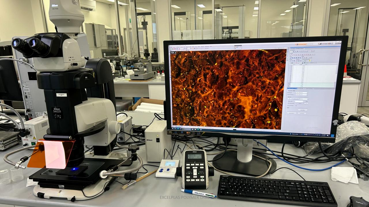
The new method using a fluorescent tracer to highlight the cracks in polymers under a UV microscope enabling greater sensitivity and contract enhancement
