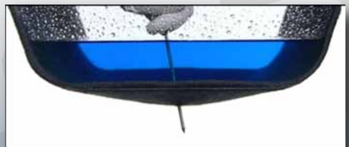
Self healing properties allow the regeneration of the seal after mechanical damage to the substrate
