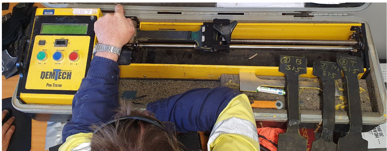
Figure 7: On-site shear tensile tests were used to confirm the good seam tensile strengths.
