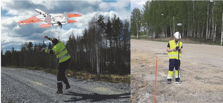
Fig. 9. Starting the fixed-wing UAV flight (left) and measuring the ground control points using a GNSS receiver (right).
