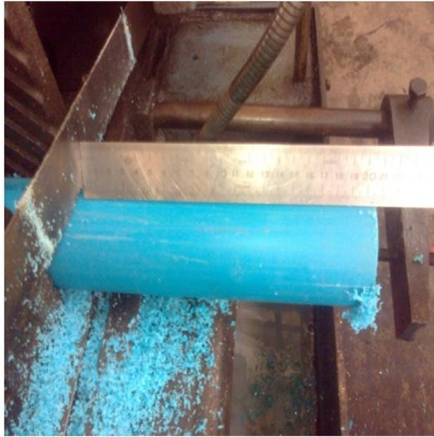
Figure 2: Measurement and cutting the required length of a pipe section.
