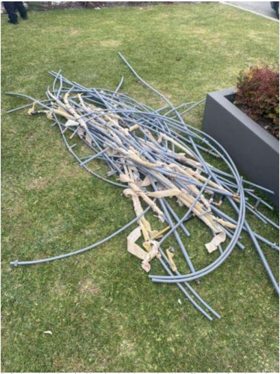
Defective polybutylene plumbing pipes have been stripped out of hundreds of new homes in WA due to water leaks and bursts that have caused huge damage NO
