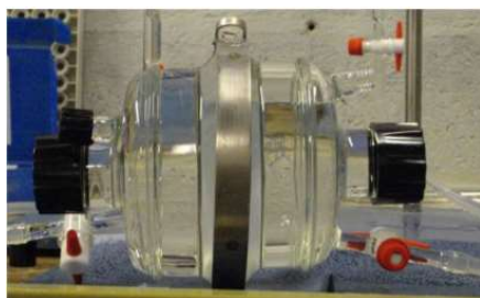
Figure 1: dual cell permeameter (overview) Photo courtesy INRAE
