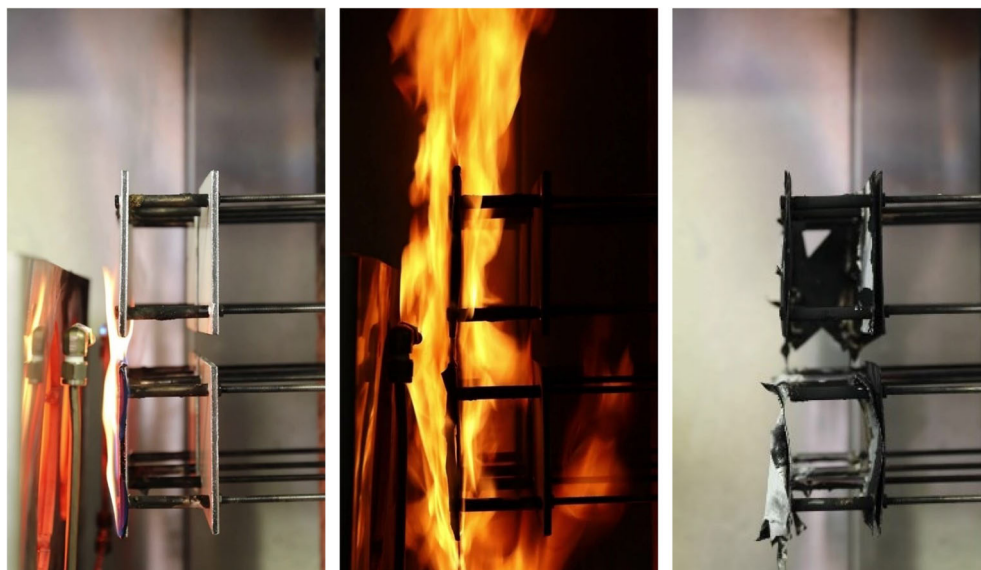
FIGURE 7 Video still captures of ACM PE experiment showing various stages in fire development; (A) ACM PE at 2 min 9 s with bottom panel burning, (B) ACM PE at 3 min 5 s with upper panel involvement, and (C) ACM PE at 9 min 24 s after burnout.
