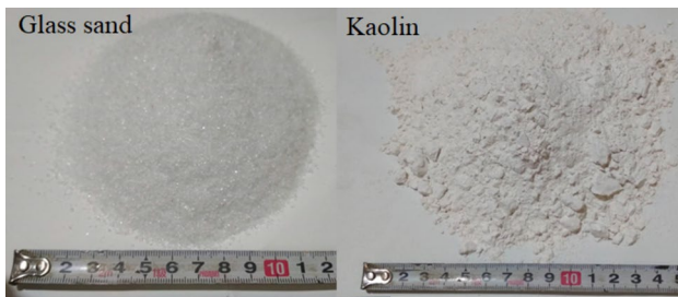
Fig. 2 Material of the surrounding rock (mixture consists glass sand and kaolin)
