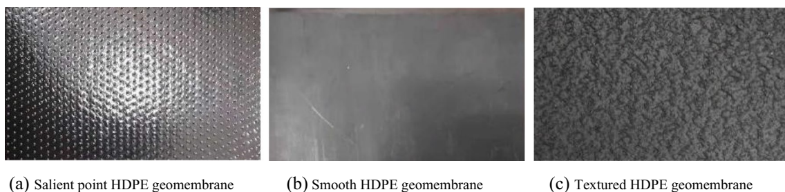
Fig. 1 Three types of HDPE geomembranes with a thickness of 1.5 mm
