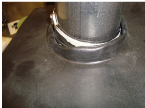
Polyethylene pipe boot pushed upwards to failure
