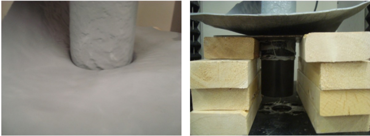
Polyurea connection pushed upwards to failure
