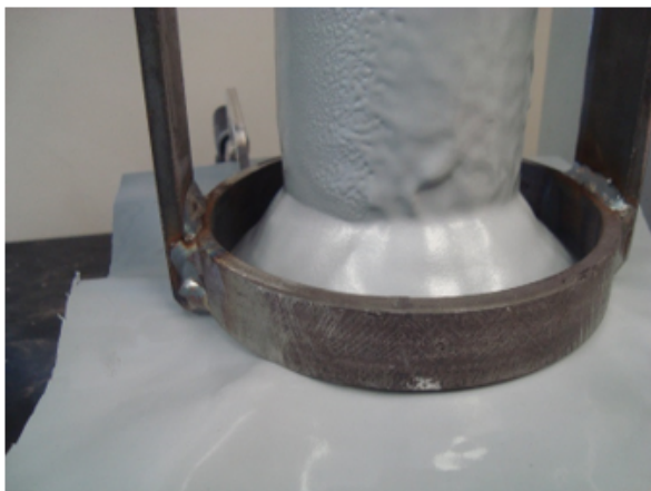
Stretching of Polyurea Boot Prior to Failure
