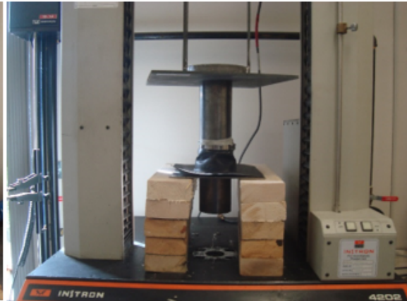
Configuration for pressing connection upward.
