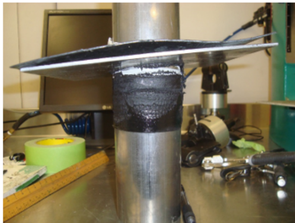
Polyethylene pipe boot pushed upwards to failure
