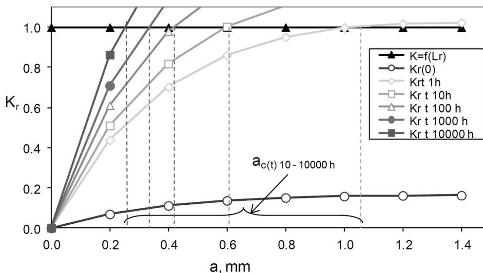
Fig. 6. The failure curves of the pipe joint with the elliptical fissure. SDR 11;  $p=0.5$  MPa;  $k=0.25$  mm;  $f=0.1$  mm;  $c=3$  mm;  $T=40^{\circ}\text{C}$
