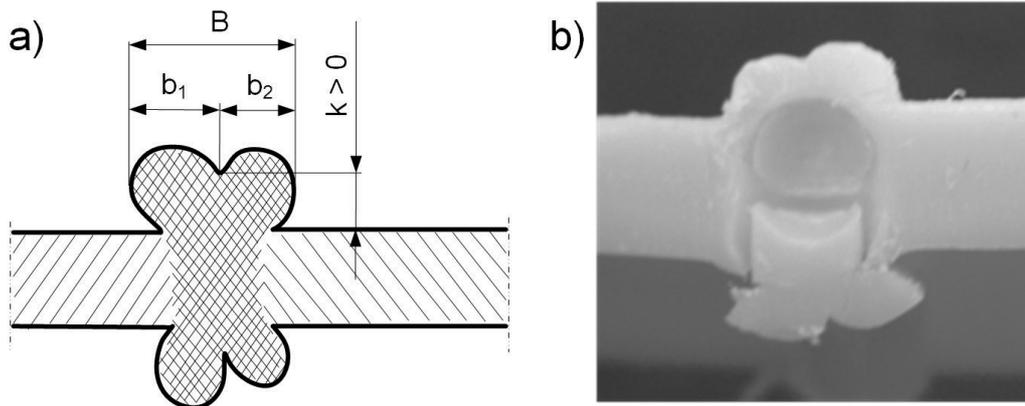
Fig. 2. Scheme (a) [3] and the view (b) of the cross-section of a butt welded joint with internal defect;  $B$  – joint width,  $b_1$ ,  $b_2$  – width of the weld beds,  $k$  – groove height between the weld beds
