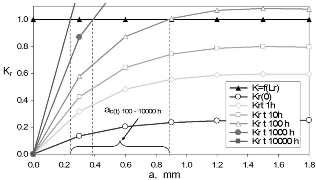
Fig. 5. The failure curves of the pipe joint with the elliptical fissure. SDR 11;  $p=1.25$  MPa;  $k=0.25$  mm;  $f=0.1$  mm;  $c=3$  mm;  $T=23^\circ\text{C}$
