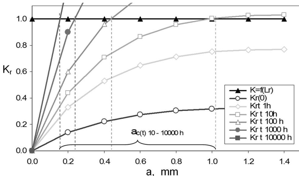
Fig. 4. The failure curves of the pipe joint with the elliptical fissure. SDR 17.6;  $p=1$  MPa;  $k=0.25$  mm;  $f=0.1$  mm;  $c=3$  mm;  $T=23^{\circ}\text{C}$
