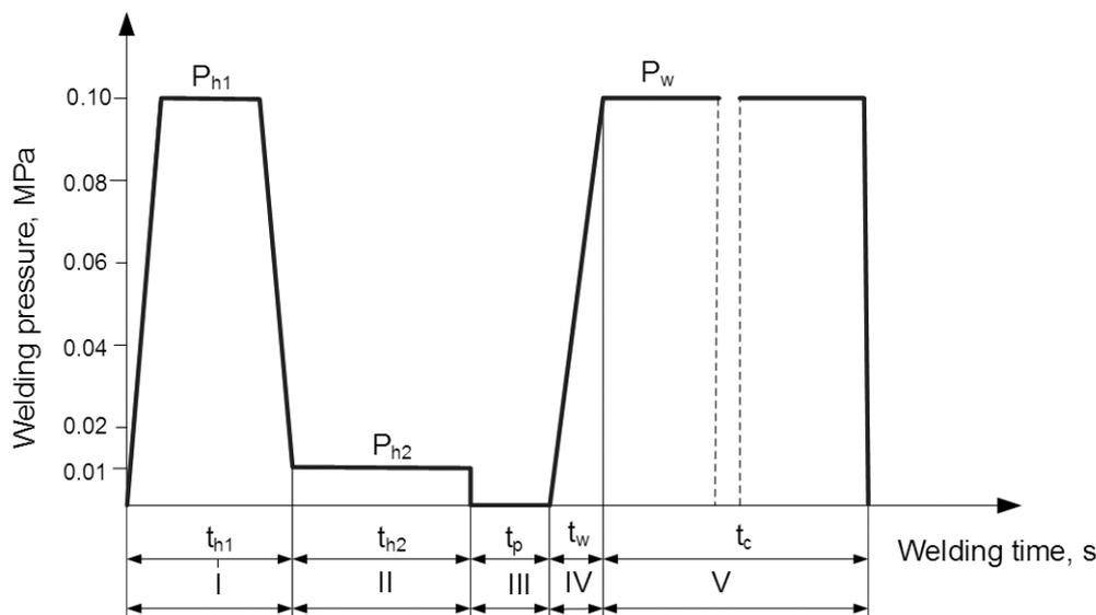
Fig. 1. The program of a welding process of thermoplastic parts with an external heating element [6,15]; description in the text
