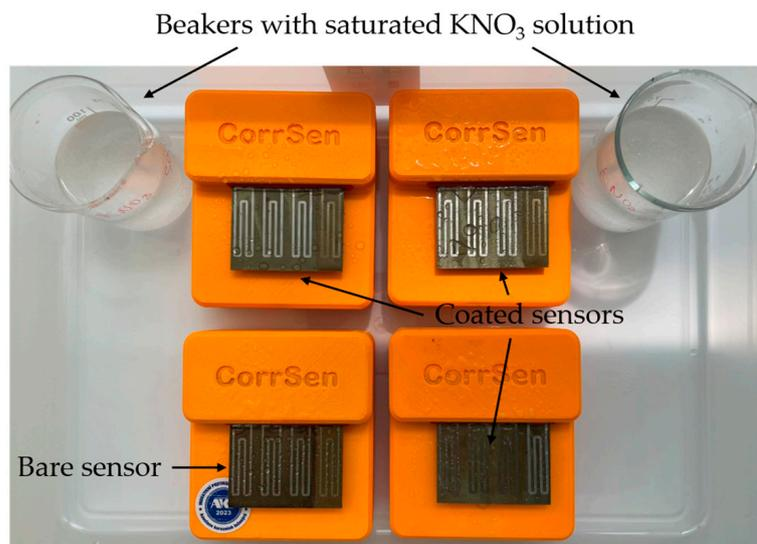
**Figure 4.** The sensors during the cyclic atmospheric test; the beginning of the wet phase after spraying with NaCl solution.
