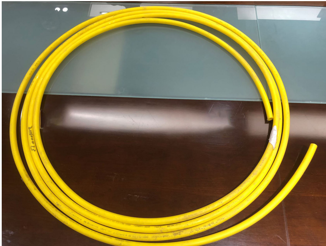
Fig. 2 Appearance of floor heating pipe
