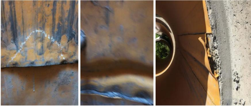
**Fig. 5** Wrinkles and panel lift-off from inadequate lacing and/or panel/tube sizing
