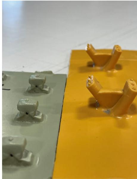
Neither of the aforementioned CPL sheets can be considered better than the other except to make your own judgment on anchor design, anchor density, and/or sheet width availability. Suregrip has 13–19 mm V-anchors at 420 anchors per square meter [2], while Studliner has 8 mm head-type anchors at 1200 anchors per square meter [6].
