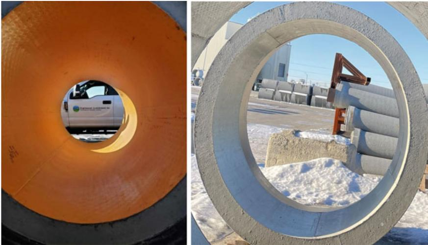
**Fig. 2** 10' width CPL on left allowing one longitudinal weld on 10' jacking pipe in the invert. The 8' width CPL on right requiring 2–3 longitudinal welds on 10' jacking pipe (3 welds are shown in the picture of 1800 mm jacking pipe)
