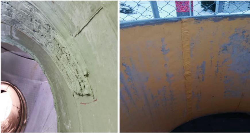
**Fig. 8** Self-performed precaster in-plant welding on left and third-party in-plant welding on right. Neither piece passed QA/QC protocols
