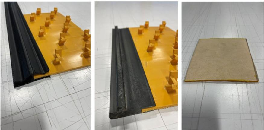
**Fig. 4** Tear-off, end, and fabric-back accessories (AGRU accessories)
