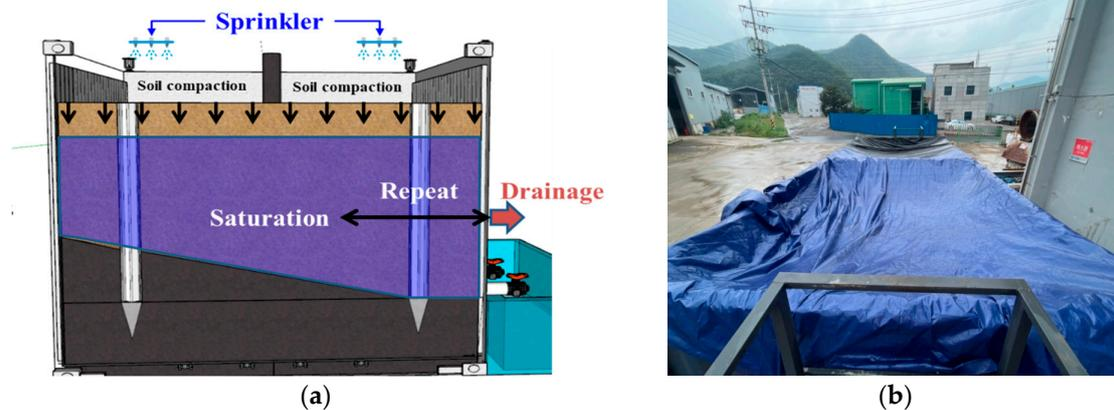
**Figure 10.** Ground stability: (a) input and discharge of water (compaction using water); (b) waterproof cover to prevent inflow of water.
