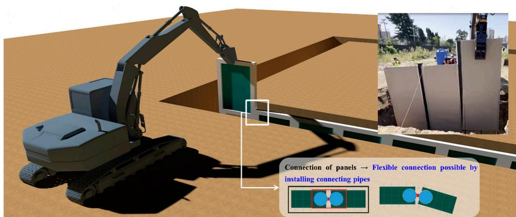
**Figure 4.** Installation of smart liner using the PIM.
