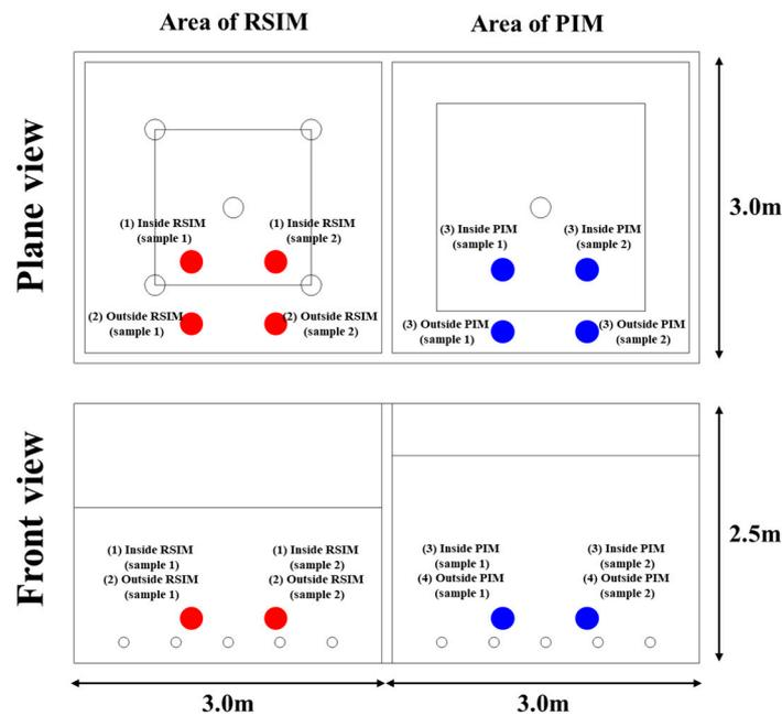
Figure 16. Locations of sample collection to check soil contamination.
