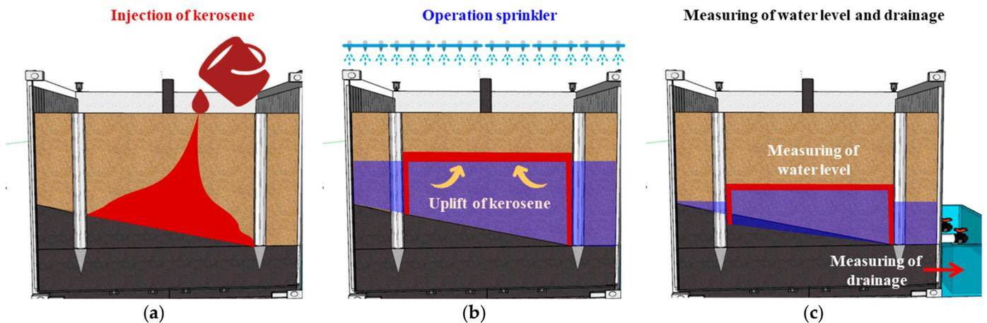
**Figure 12.** Experimental procedure for verifying the performance of smart liner with TPH injection: (a) injection of TPH (procedure 1); (b) operation of sprinkler (procedure 2); (c) measurement of water level and drainage (procedure 3).
