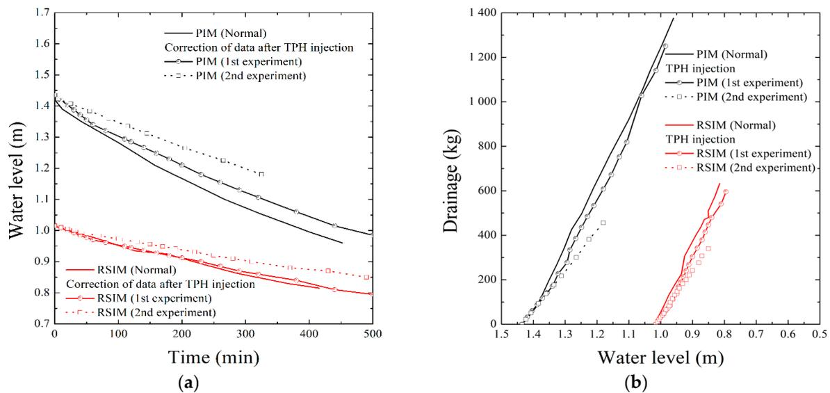
Figure 15. Data correction after TPH injection: (a) water level with time; (b) drainage with water level.
