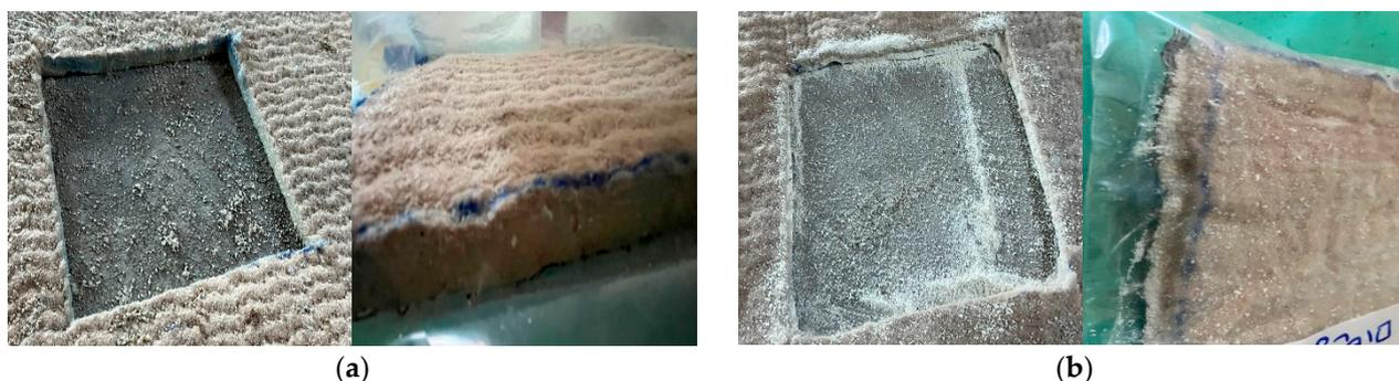
**Figure 18.** Inspection of reacted areas: (a) gelation of the smart liner; (b) powder form of the smart liner.
