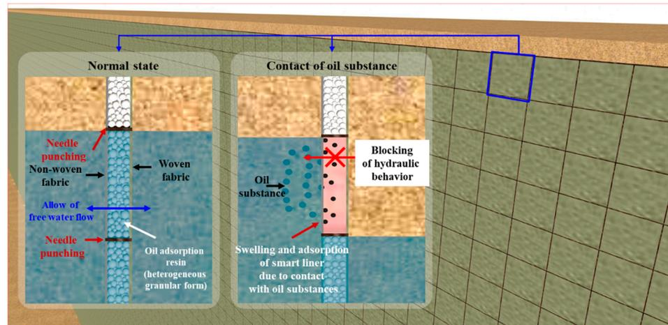
Figure 1. Smart liner for preventing oil spills on the ground.
