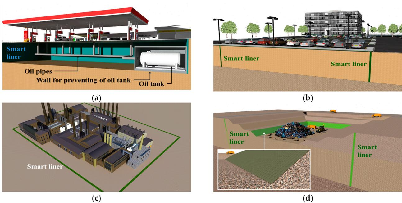
Figure 2. Applications of smart liners: (a) oil station; (b) parking lot; (c) oil refinery; (d) landfill.
