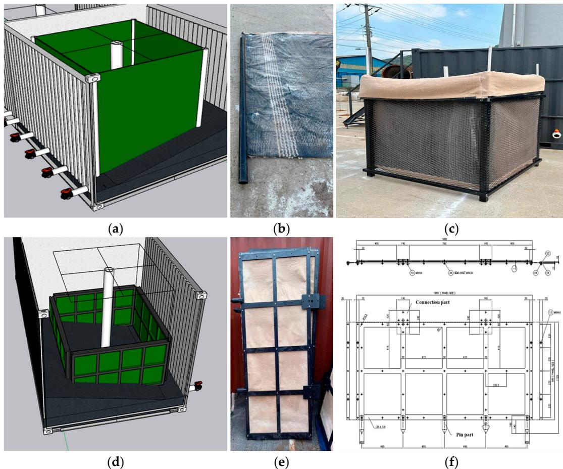
**Figure 7.** RSIM: (a) installation schematic; (b) connection of supporting pile and smart liner using connecting pipe; (c) outside frame to support the weight of smart liner; and PIM: (d) installation schematic; (e) connection of panel and smart liner; (f) design drawings of the modular panel.
