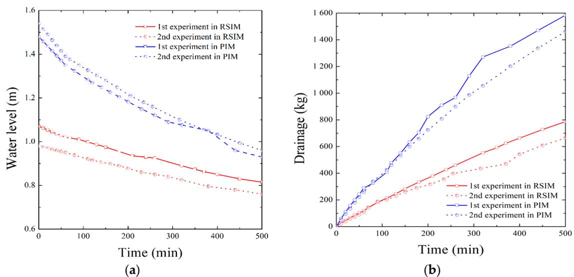
**Figure 13.** Ground stability over time: (a) water level; (b) drainage.
