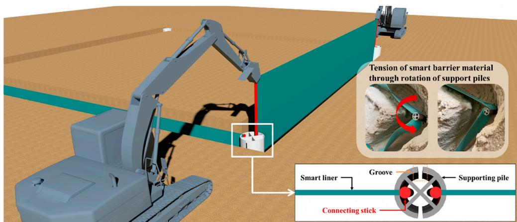
**Figure 3.** Installation of smart liner using the RSIM (modified from [34]).
