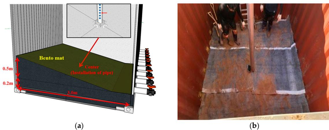
**Figure 6.** Subground and observation pipe: (a) installation schematic; (b) composition of subground, slope, and observation pipe.
