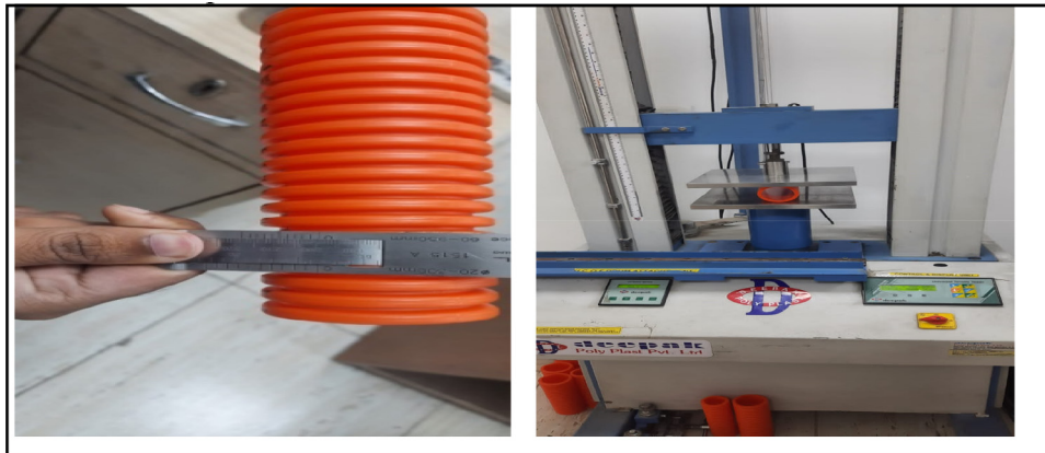
Fig. 6. HDPE pipe diameter measurement and Compression testing.
