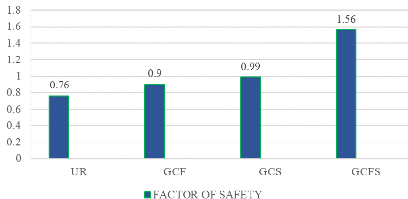
Fig. 10. Variation of factor of safety for different configurations of the slope
