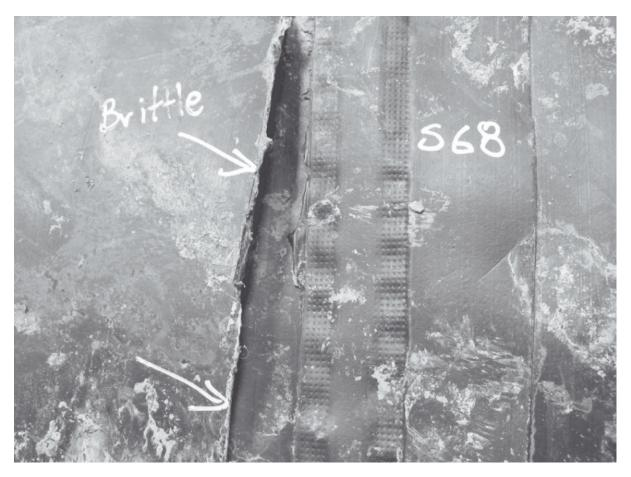
Stress Crack Resistance (SCR) – Key to Weld Ductility and Durability
