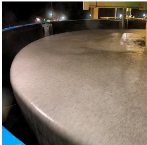
Figure 8. Concentrate overflowing a HydroFloat cell at Cadia
